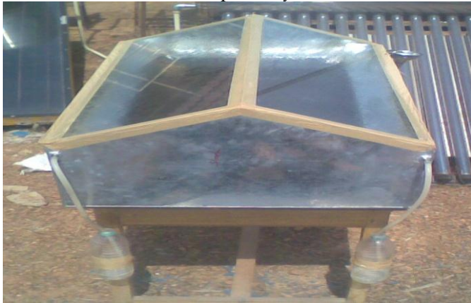
Fig 2.1: Solar still without PCM
